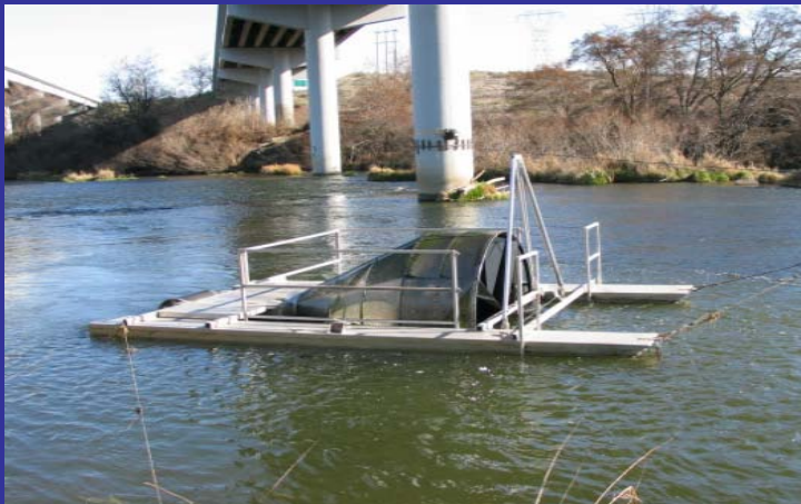
Screw trap for outmigrant capture
